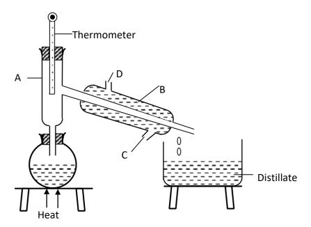
(b) Name the piece of apparatus labelled B. (1 mark)
