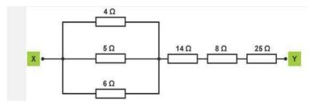
i) Determine the total resistance in the circuit between X and Y
